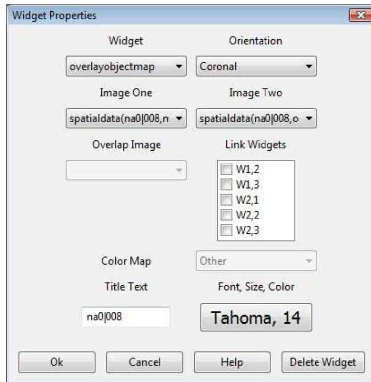
Figure 3.9: PanelForm GUI. The PanelForm GUI allows the user to make changes to the current Panel. The user can change the view/widget, the orientation, the input images, the color map, the title of the Panel, and even the attributes of the title.
