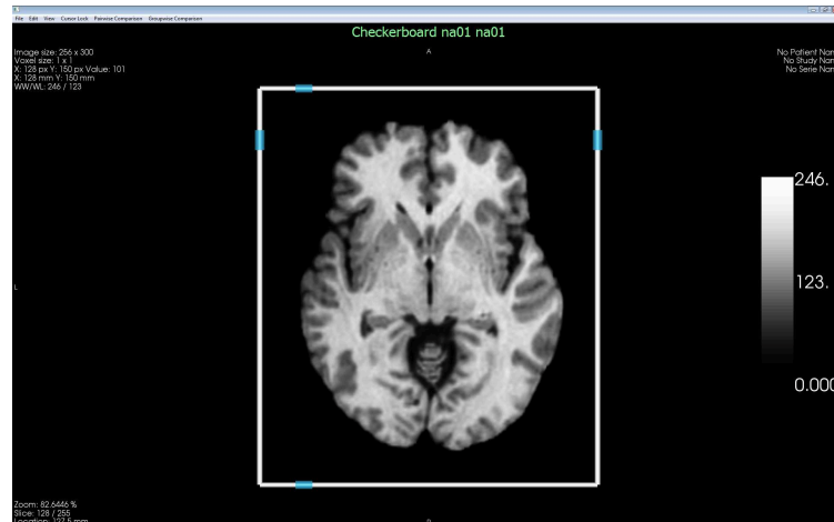
Figure 3.1: Checkerboard view widget, of two images na01 and na01. This is showing when two images align perfectly, the checkerboard view widget will look like one image.
